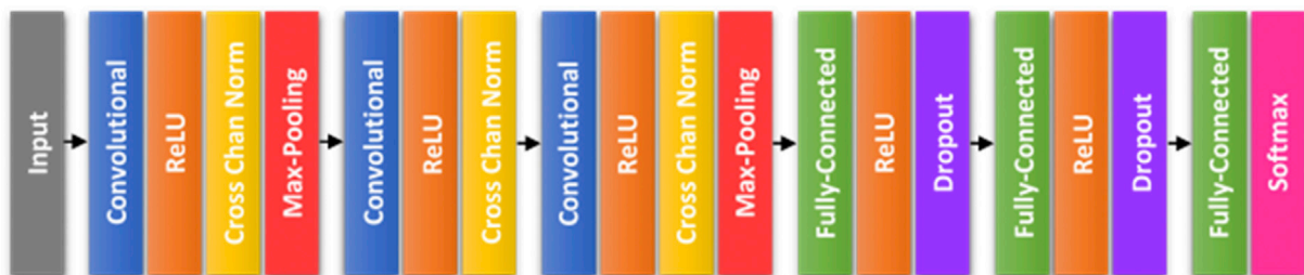
Fig. 5. Layers of proposed CNN architecture.
